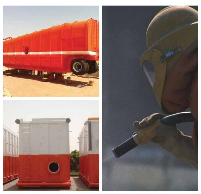
Blasting is a process of cleaning and finishing in metal by forcefully using abrasive media against the surface of metal. Blasting makes an old metal new by removing dust and impurities. On the other hand painting is a process which increases the durability of the metal. It can be either mid coating painting (up to 400 microns) or final coating (up to 70 microns)
