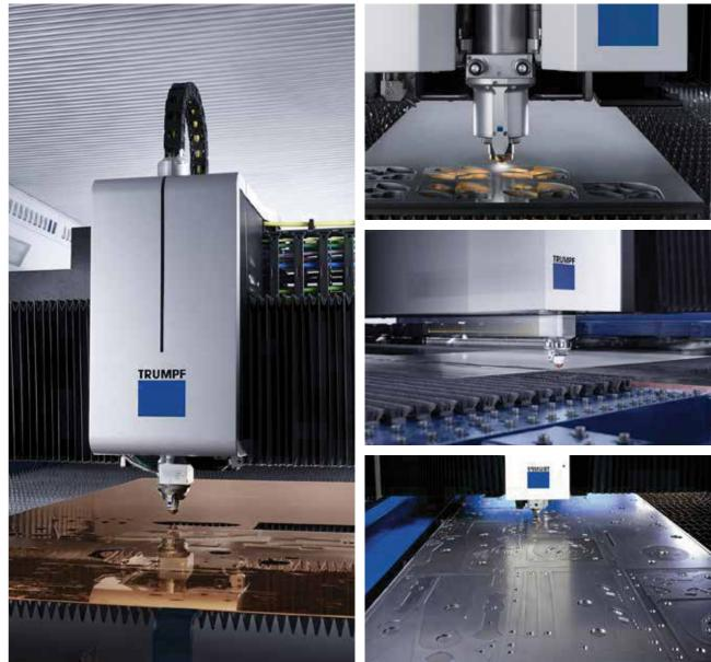
Laser cutting is a technology that uses a laser to cut materials, and is typically used for industrial manufacturing applications : a laser is a device that generates an intense beam of coherent monochromatic light used in drilling and cutting, alignment and guidance.
