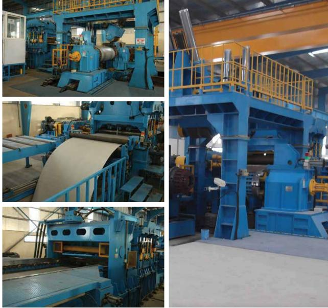
A flat sheet of material is not actually produced by a mill as a flat sheet. In reality, a flat sheet of material starts its life as part of a coil of material. A Cut-To-Length machine will uncoil the material, level it, and then cut it to the required length and stack it. The end product produced by a Cut-To-Length machine is a flat sheet of material cut to a very precise length tolerance.
