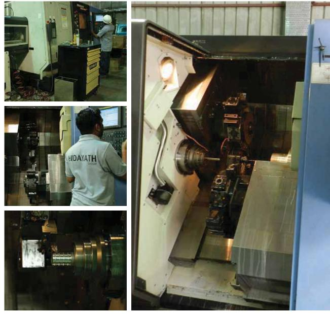
A lathe is a tool that rotates the work piece about an axis of rotation to perform various operations such as cutting, sanding, knurling, drilling, deformation, facing, turning, with tools that are applied to the work piece to create an object with symmetry about that axis. A chuck is a specialized type of clamp. It is used to hold an object with radial symmetry, especially a cylinder. On a lathe the chuck is mounted on the spindle which rotates.
