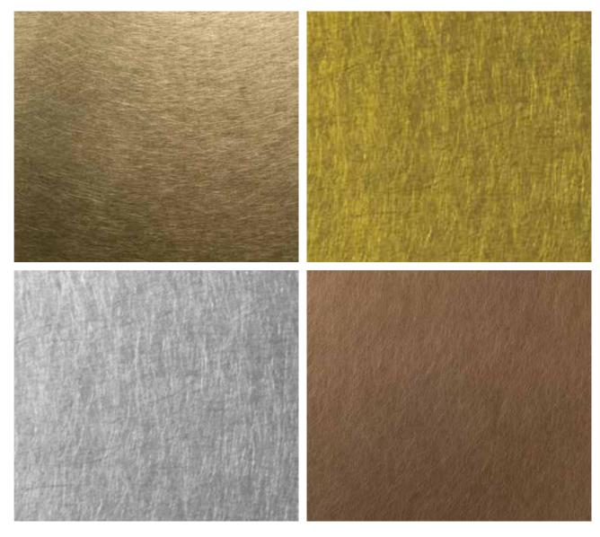
This is a non directional, non uniform finish made by vibrating rough abrasives that embed multiple continuous scratches overlapping each other. This is one of the popular finishes and could be called modern art on stainless steel.
