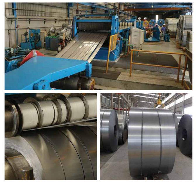
Slitting is used to cut a wide coil of metal into a number of narrower coils as the main coil is moved through the slitter Also referred to as a type of metal cutting process where large rolls, or coils, of sheet metal stock are cut using extremely sharp rotary blades.
