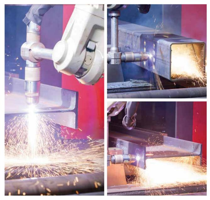
**Bolt Holes** – High quality, AISC compliant, in unlimited sizes with no tool changeovers; PythonX tilts the cutting torch, instantaneously changes speeds and uses sophisticated software to produce straight through holes that are nearly Taperless.
