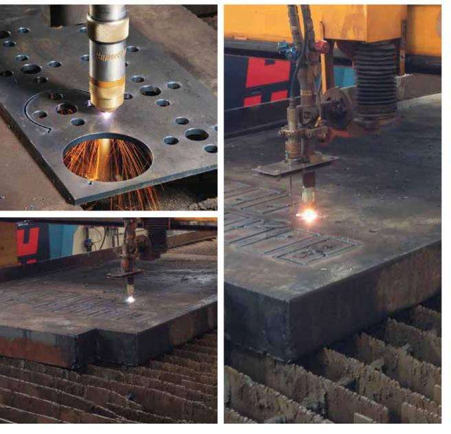
Oxy fuel cutting use a combination of fuel gases and oxygen to cut metals. Suitable for medium-sized and thick materials. Economic use of several torches. Low investment and consumables costs. Bevel cutting with up to three torches on one aggregate.
