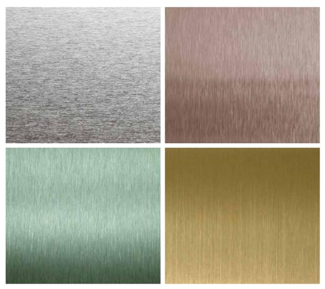
Also known as brushed, directional or satin finish. A #4 architectural finish is characterized by fine polishing grit lines that are uniform and directional in appearance. It is produced by polishing the metal with a 120–180 grit belt or wheel finish and then softened with an 80–120 grit greaseless compound or a medium non-woven abrasive belt
