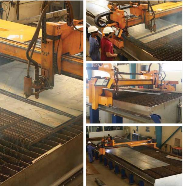
Plasma cutting is a process that cuts through electrically conductive materials by means of an accelerated jet of hot plasma. Plasma – a fourth state of matter which is ionized gas, it occurs when gas is heated at a very high temperature (20,000 deg. Cent.) And achieve equal number of positively charged ions and negatively charged ions. So under plasma cutting machine the gas is of high temperature and pressure. Thus it can only be used on high temperature and pressure.
