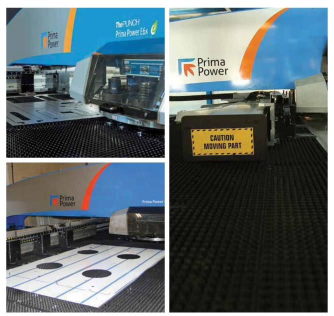
Punch presses are developed for high flexibility and efficient processing of metal stampings. The main areas of application are for small and medium runs. This method is used where the application of lasers are inefficient or technically impractical. Punching is often the cheapest method for creating holes in sheet metal in medium to high production volumes. When a specially shaped punch is used to create multiple usable parts from a sheet material the process is known as blanking.
