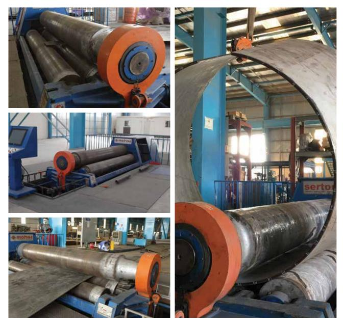
In metalworking, rolling is a metal forming process in which metal stock is passed through one or more pairs of rolls to reduce the thickness and to make the thickness uniform. The concept is similar to the rolling of dough. A plate rolling machine is a machine that will roll different kinds of metal sheet into a round or conical shape. It can be also called a "roll bending machine", "plate bending machine" or "rolling machine.
